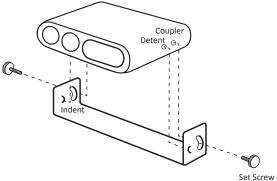
Detent on transponder lines up with indent on the bracket. Position is locked into place with the set screw.
