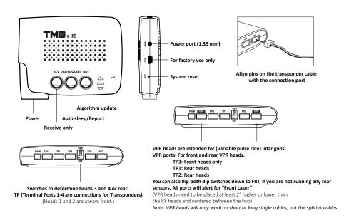
The RDT port is for radar detector integration, or other accessories. The side PWR port can be used to power the unit with a 12v barrel connector 1.3 mm.
